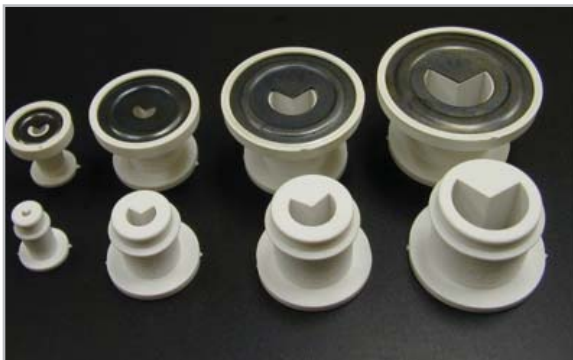
Representative "doodads" and "gadgets" used as chip defectors during the gundrilling operation. Available from Star SU.
